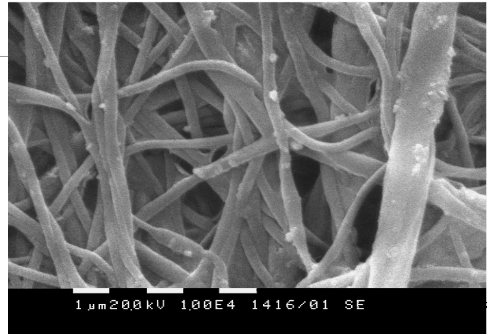
PCL/AP(30%) fibers after a 6-h stay in aqueous solution of AgNO 3
